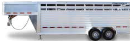
Model 8117. Model 8117 livestock trailer is a great value and option for your livestock hauling. It is available in 16', 20' and 24' lengths and is 6'7" wide. It has an aluminum floor standard with a full-swing rear gate with lockable slider.
