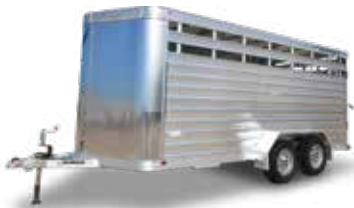
Model 8107. Bumper pull stock trailer with aerodyne nose features a gravel guard standard. Available in heights of 6'6", 7'0" or low profile 5'3". Length options include 12', 16' or 20'.
