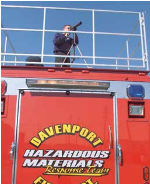
Observation decks offer additional space for assessing an emergency
