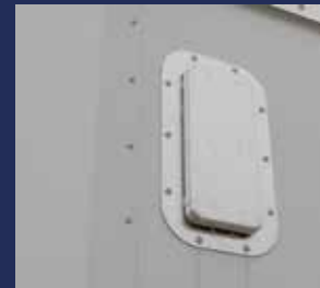
Streetside Air Vent
